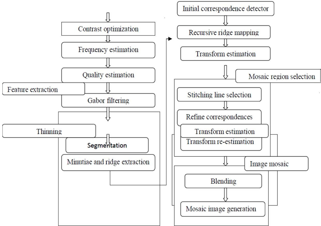
**Fig.3.1.1** Showing the Process flow of Mosaic Slice based Architecture.
