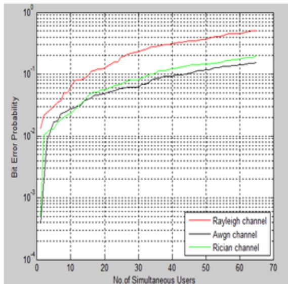
**Fig.4.1** BEPs of our Two\_level FH-CDMA scheme under AWGN, Rayleigh and Rician Fading channels.
