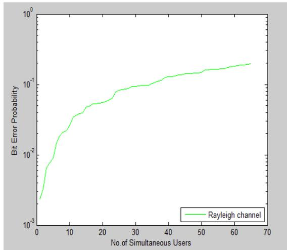
**Fig 3.1.1** BEP of Rayleigh Channel using Bi-level FH-CDMA for No. Of simultaneous users.
