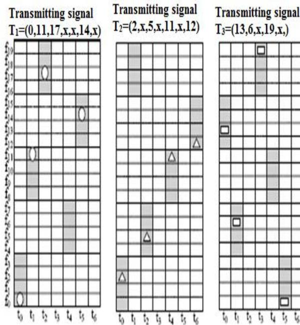
**Fig.2.1.1** Example of the encoding process of the two-level FH-CDMA scheme with three simultaneous users.
