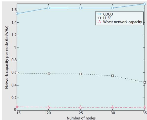
**Fig.4.1** Network capacity versus different numbers of nodes in the MANET.
