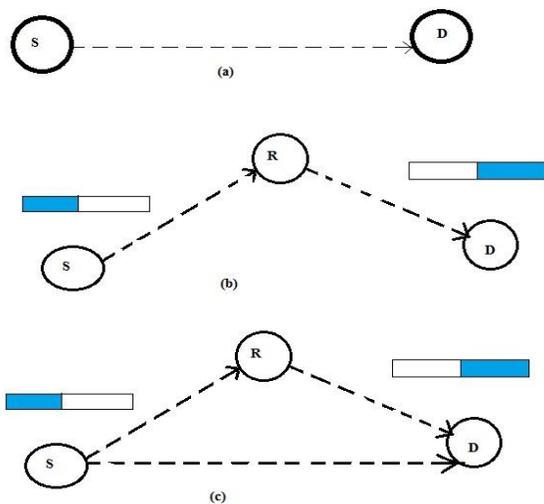
**Fig.2.1.1.** Three transmission protocols: a) direct transmission via a point to point conventional link. b) Multi – hop transmission via a two- hop manner occupying two time slots. c) Cooperative transmission via a cooperative diversity occupying two
