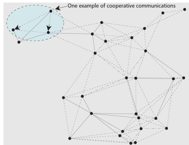
**Fig.3.2.2** The final topology generated by COCO. The solid lines denote traditional direct transmissions and multihop transmissions. The dashed lines denote the links involved in cooperative communications.
