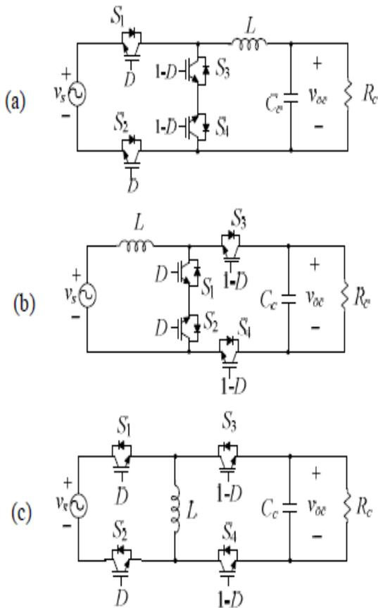
**Fig.2.3. The single-phase Ac-chopper converters; (a) buck, (b) boost, (c) buck-boost types.**
