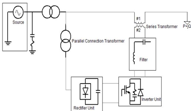
**Fig. 2.4 Series and Parallel Connection Block DVR**
