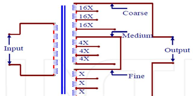
**Fig. 3.1 Changing Switch Arrangement in offload**
