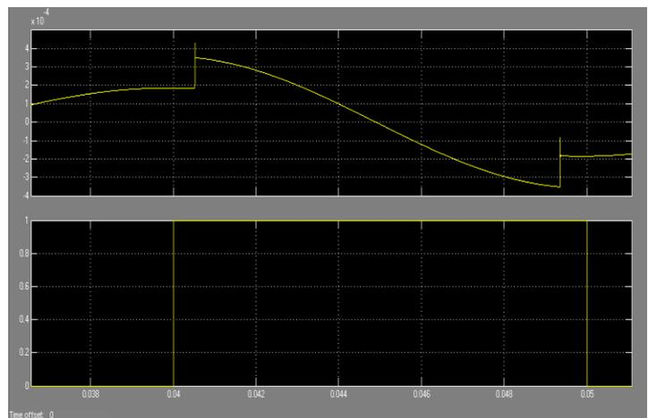
Fig. 5.4. The simulated waveforms when voltage sag occurs, (upper) error voltage,  $v_e$ , (bottom)  $u_{ty}$  ratio,  $D$ .
