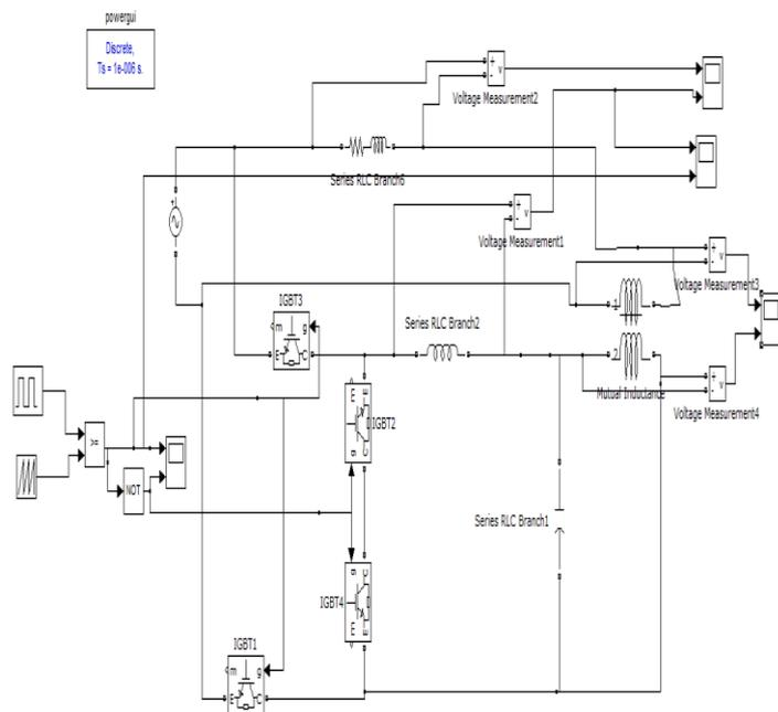
**Fig.4.2 . The DVR system with a buck ac-ac converter.**
