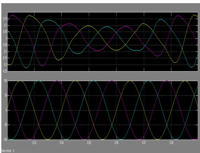
**Fig. 5.7. The simulated waveforms when voltage sag occurs, (top) three p hase input voltages,  $v_{sa}$ ,  $v_{sb}$ ,  $v_{sc}$  with 20% sag, (bottom) three phase .load voltages,  $v_{oa}$ ,  $v_{ob}$ ,  $v_{oc}$ .**
