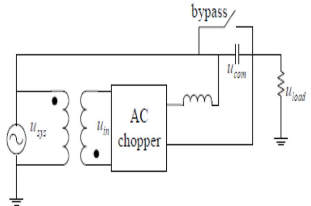
**Fig. 2.5 Principle Block Diagram of AC-Chopper**
