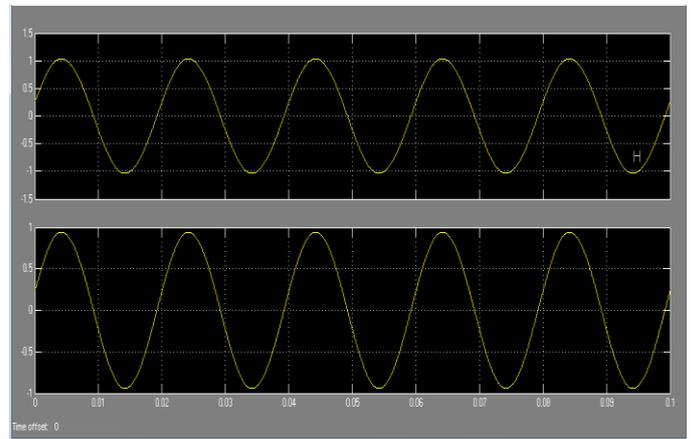
Fig. 5.3. The simulated waveforms when voltage sag occurs, (upper) input voltage,  $v_s$  with 30% sag, (bottom) load voltage,  $v_o$ .
