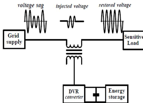
**Fig 1.1 Principle of operation of the dynamic Voltage Restorer**
