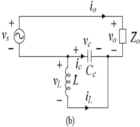
**Fig. 4.3** The equivalent circuits (a) during  $DTs$ , (b) during  $(1-D)Ts$
