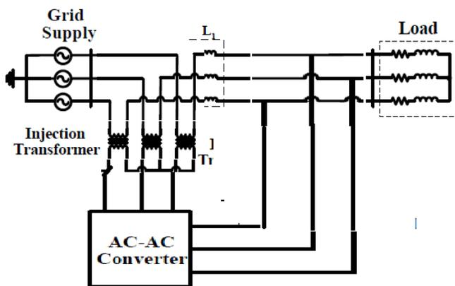
Fig.2.2 The proposed Ac-chopper converter; (a) shunt series, (b) series-shunt configurations.
