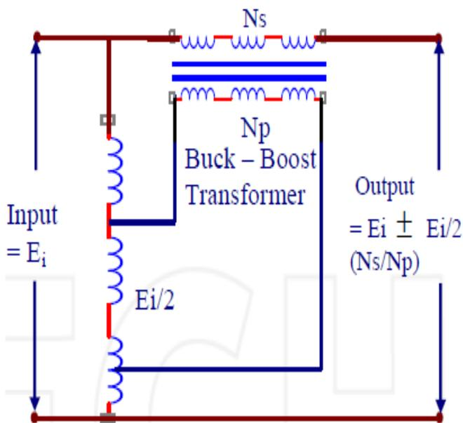
**Fig. 3.2 Voltage control by combination of a Buck-Boost transformer and a variac**
