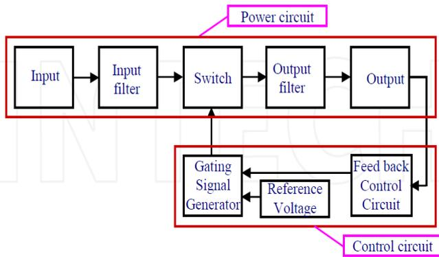
Fig. 2.1 shows the system configuration of the proposed Ac-chopper converters.
