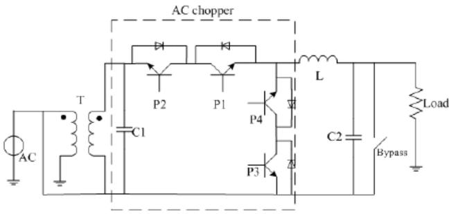
**Fig. 2.6 AC-Chopper Circuit Structure**
