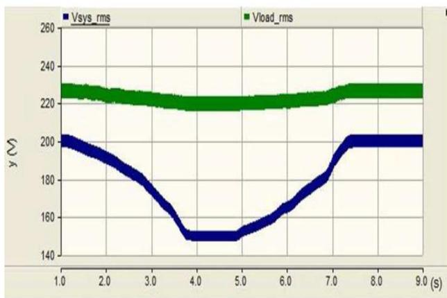
**Fig. 5.1 Green line: Voltage on load side/Blue line: System voltage wave form**
