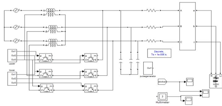
**Fig. 5.2 . The proposed series-shunt three-phase DVR using three-phase PWM ac-ac converter.**
