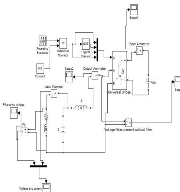
**Fig: 4.1 Simulation of a 2 level (SPWM) inverter**
