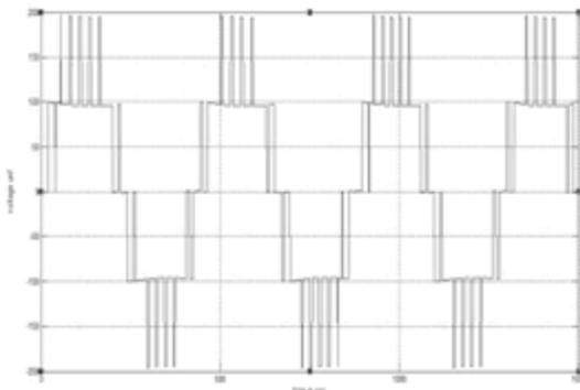
**Fig:6.4 Filtered 2 level output voltage waveform**
