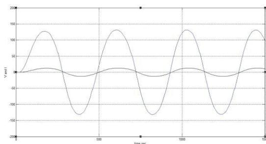
**Fig:6.5 Both voltage and current waveforms of 5 level inverter**
