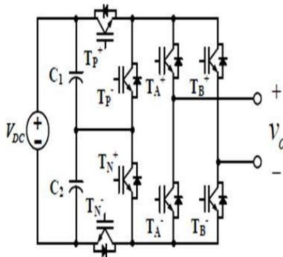
**Figure 3.1.2: Proposed Five Level H-Bridge Inverter**
