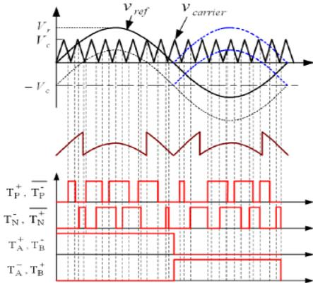
Figure 3.1. PWM strategy based on POD with carrier signal
