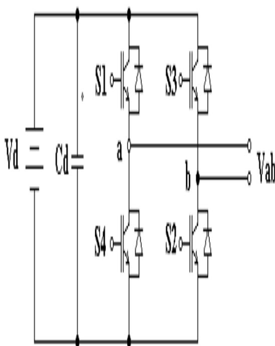
**Fig.2.1: Single Phase H- Inverter**
