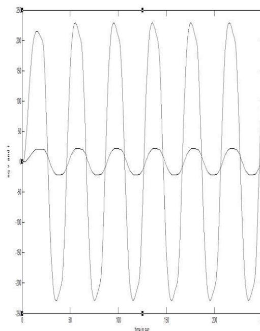
**Fig:6.1 Both voltage and current waveforms of 2 level inverter**
