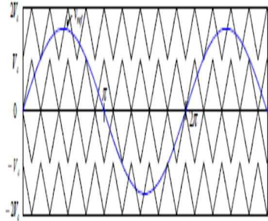
**Fig. 3.1.4 Carrier and reference signal arrangements for phase opposition and disposition**
