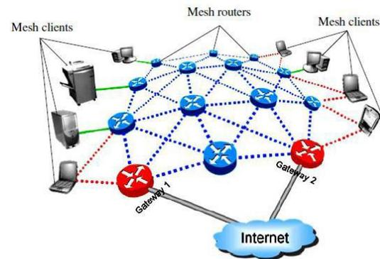
**Figure 1: Wireless Mesh Network Infrastructure**
